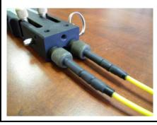
Using a standard cap crimping tool, crimp the Shock Tube into the FAST Initiator about an inch above the green plastic nut.
