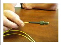
Depending on how tightly you crimp, the Shock Tube may or may not stay attached upon firing.
