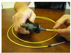
Has standard 7/16" diameter by 20 threads per inch, common to most firing devices, including the Omni devices and the MK54.
