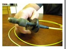
Make sure the internal threads on you firing device are clean before using.
