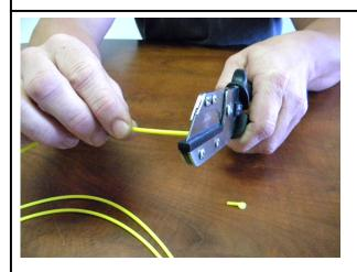
Cut or trim the Shock Tube with a razor or sharp knife. Do not use fuse crimpers for cutting as they may close the end of the tube.
