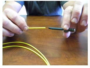
Insert the trimmed end of the Shock Tube into the open end of the FAST Initiator. The tube should be pushed all the way into the initiator.
